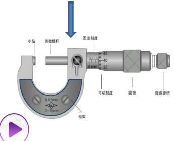
This microcalliper is used to measure the thickness of plastic tape and plastuic bags,if you have no idea of the method how to use it,you can click the left botton to learn.
